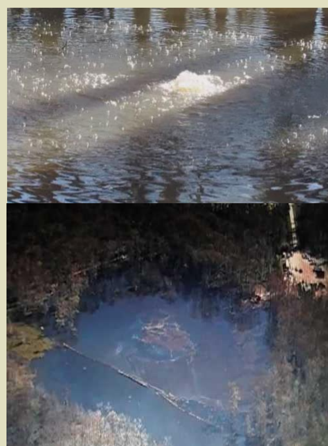
Figures 1 A/B. Examples of excessive methanogenesis (top panel – A) and associated ebullition/induced migration of contaminants yielding a sheen (bottom panel – B)
