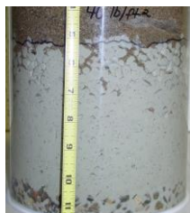
Photo 4. 3070 SW Clay Blend, 40lbs/SF (immediate load).
