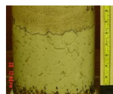
Photo 6. 4060 SW Attapulgite, 30lbs/SF (immediate load).
