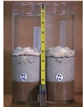
Photo 2. Attapulgite-Based Product Hydrated in fresh (left) versus high saline waters (right).
