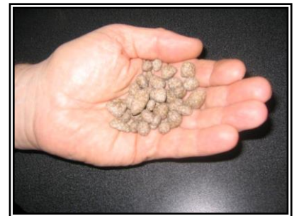
Figure 3. AquaBlok HoleBlok™ and HoleBlok+™ grout particles are easy to handle and place. No mixing or special equipment is required.
